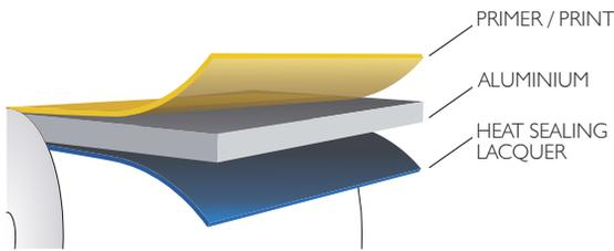
We supply lacquered hard tempered **lidding foil**, suitable for printing and sealing to base materials such as PS, PVC, PVDC.
