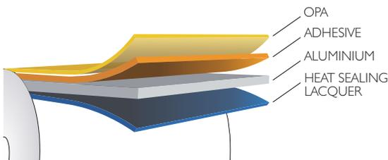
We developed a specific laminated foil, composed of **OPA/AL/Heat Sealing lacquer**, to manufacture tropical coldform with even higher protection against temperature and moisture.
