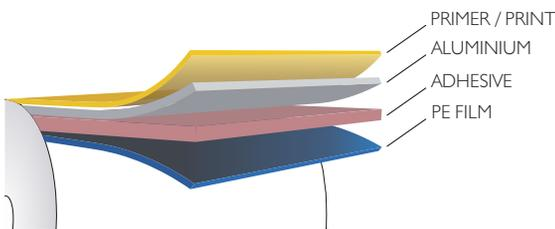
We provide laminated foil **AL/PE** suitable for strip and suppository packaging. The material can be printed and sealed on itself. This solution guarantees high seal integrity and good mechanical properties.
